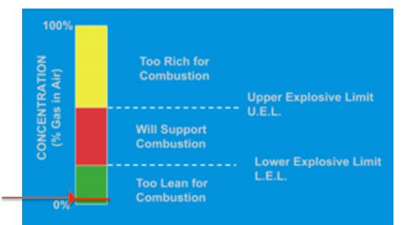
10% of LEL for Methane ( $CH_4$ ) is 0.5% gas 10% of LEL for Propane ( $C_3H_8$ ) is 0.215% gas
